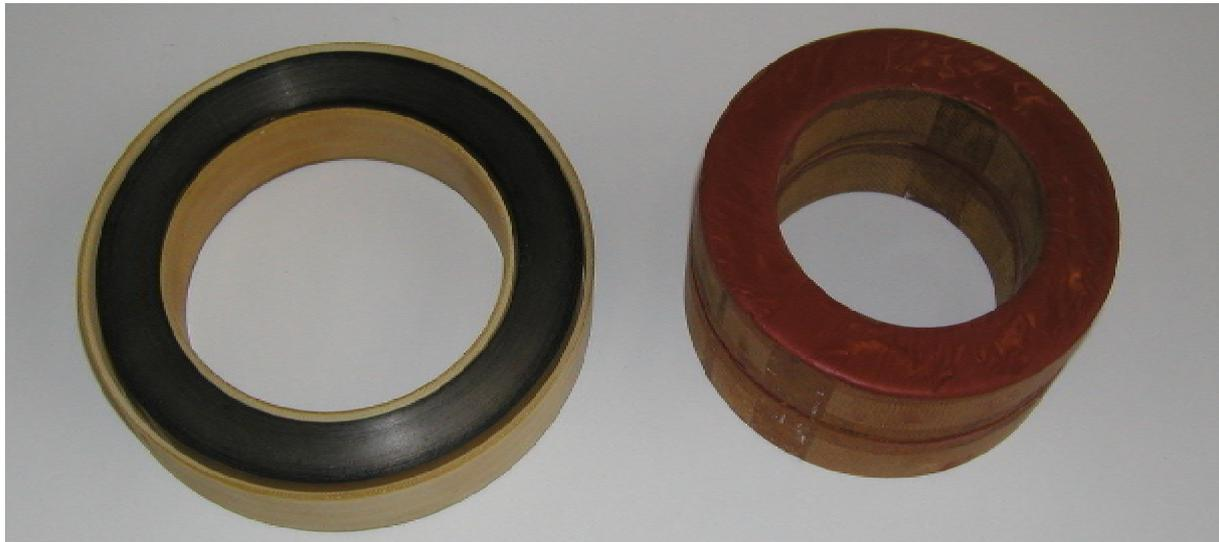
*Fig. 3: Nanocrystalline core before (left) and after filling (right).*
